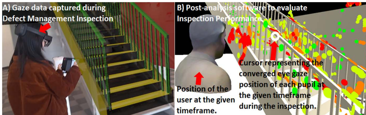
Figure 1: (Left) The inspector conducting a defect management inspection of a building using an experimental AR system. (Right) the presented gaze-based data analysis tool is used to playback the inspection for performance evaluation and analysis.
