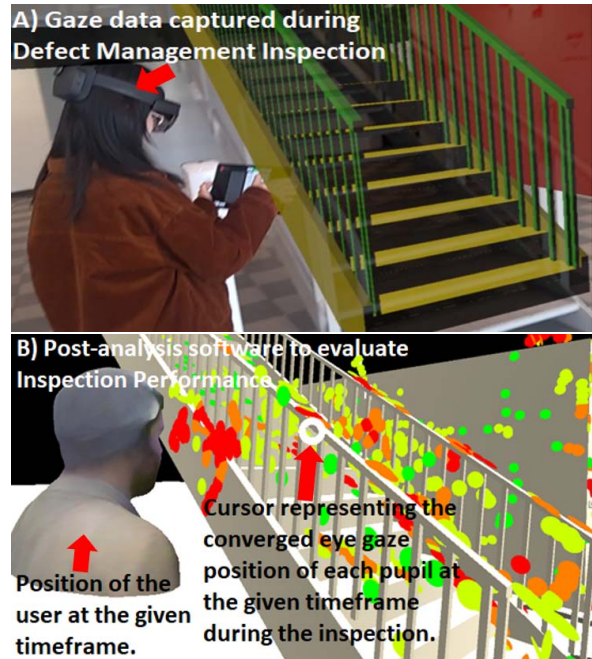
Figure 3: This figure demonstrates the playback visualisation of an on-site inspection. The top image shows a user conducting a DM inspection of the building. The bottom image shows the 4D playback visualisation of the DM inspection.
