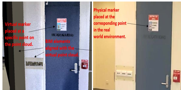
Figure 2: This figure shows the process of calibrating the virtual BIM model with the physical building/construction site. The left image shows a virtual marker placed at a specific location on the BIM model. The right image shows a physical marker placed at the corresponding location in the real-world environment.
