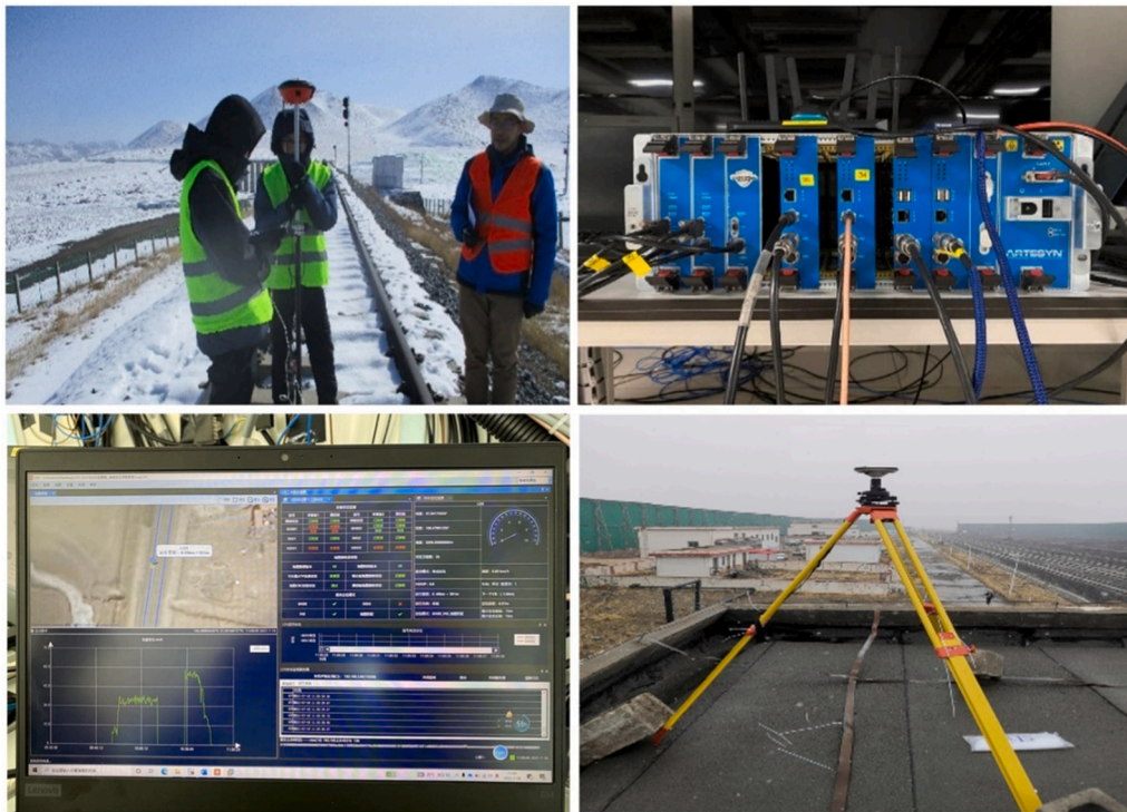
Fig. 9. Trackmap generation and equipment deployment in field test in Haergai-Muli railway.
