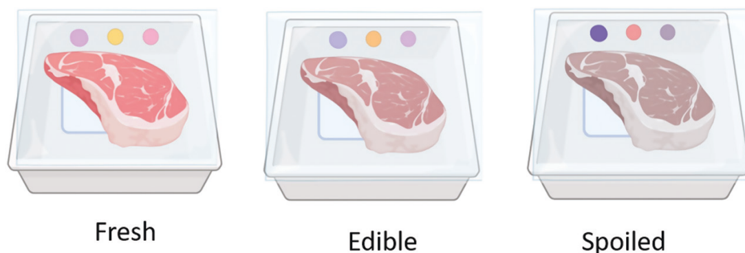
Figure 8. Example of on-pack labels that could be applied to modified atmosphere packaging for real-time quality indication and direct consumer interpretation.
