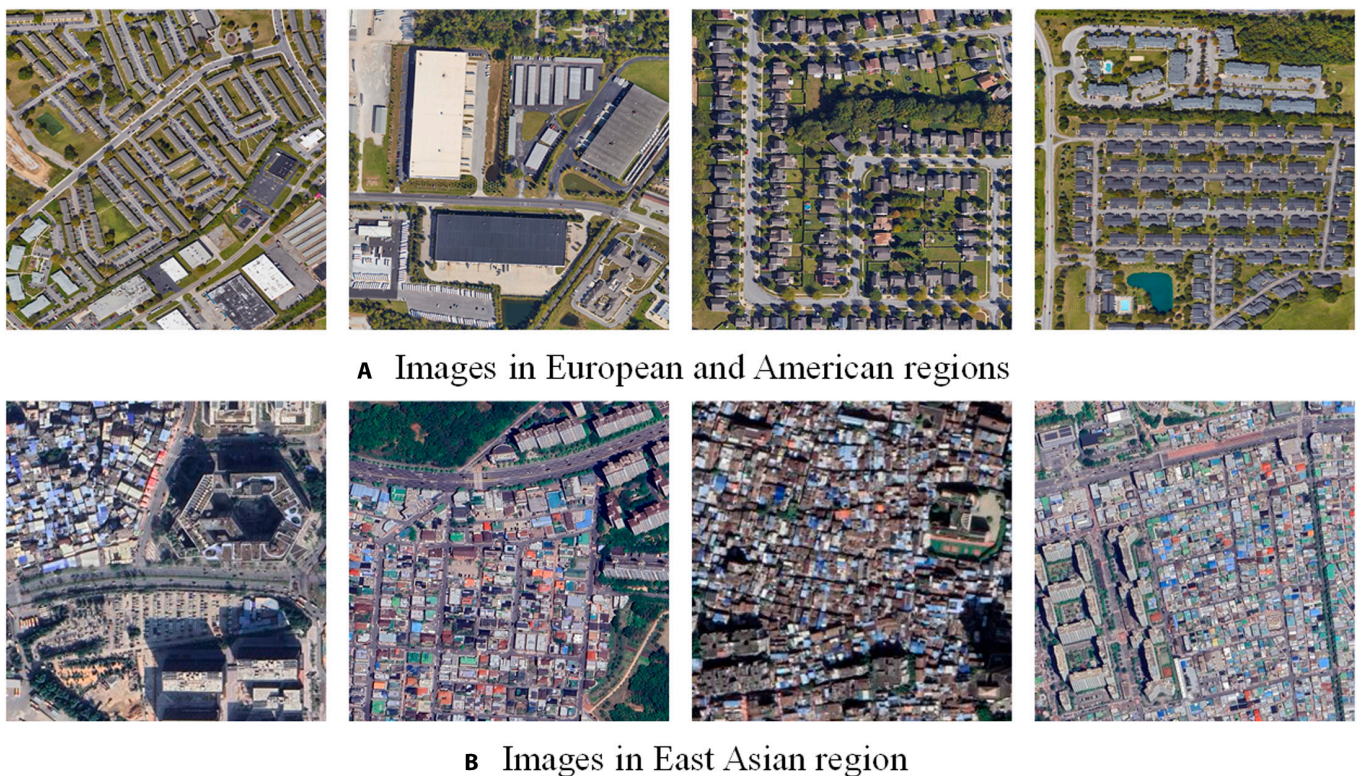
Fig. 2. Google Earth images with different resolution in different regions. (A) European and American regions. (B) East Asian regions. The images show the relatively poor quality of the images in East Asia. The visual sharpness and spatial resolution of some images in East Asia look inconsistent, which may be obtained by resampling. These images are not helpful for precise building extraction. Images are from © Google Earth 2021.
