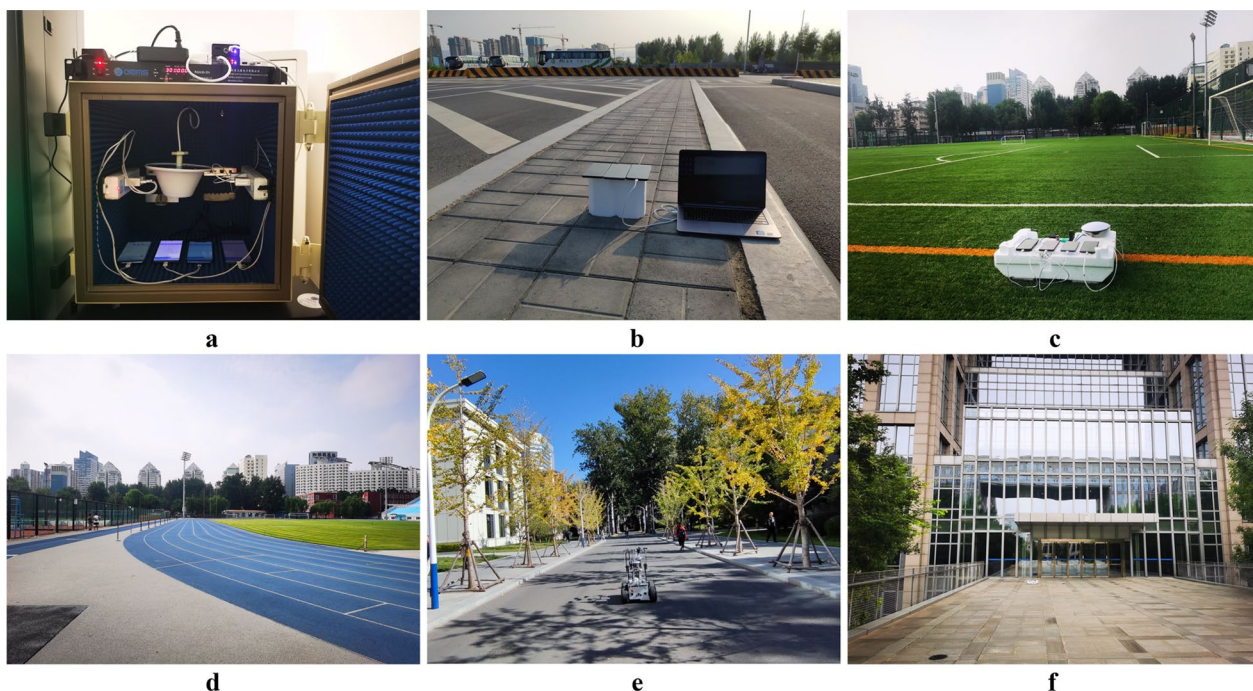
Fig. 7 Experimental scenarios under different test conditions. a Experiment 1—observation noise analysis under zero baseline condition b Experiment 2—TTFB comparison in areas with good cellular signal quality c Experiment 3—static positioning test under open sky d Experiment 4—kinematic positioning test under open sky e Experiment 5—kinematic positioning test in realistic environment f Experiment 6—3DMA GNSS positioning exploration in challenging urban area
