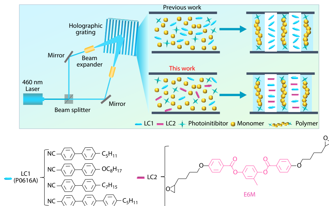
Fig. 1 Schematic illustration on the construction of high-performance LC-based holographic polymer nanocomposites by doping E6M. P0616A was commercially available LC in nematic phase.
