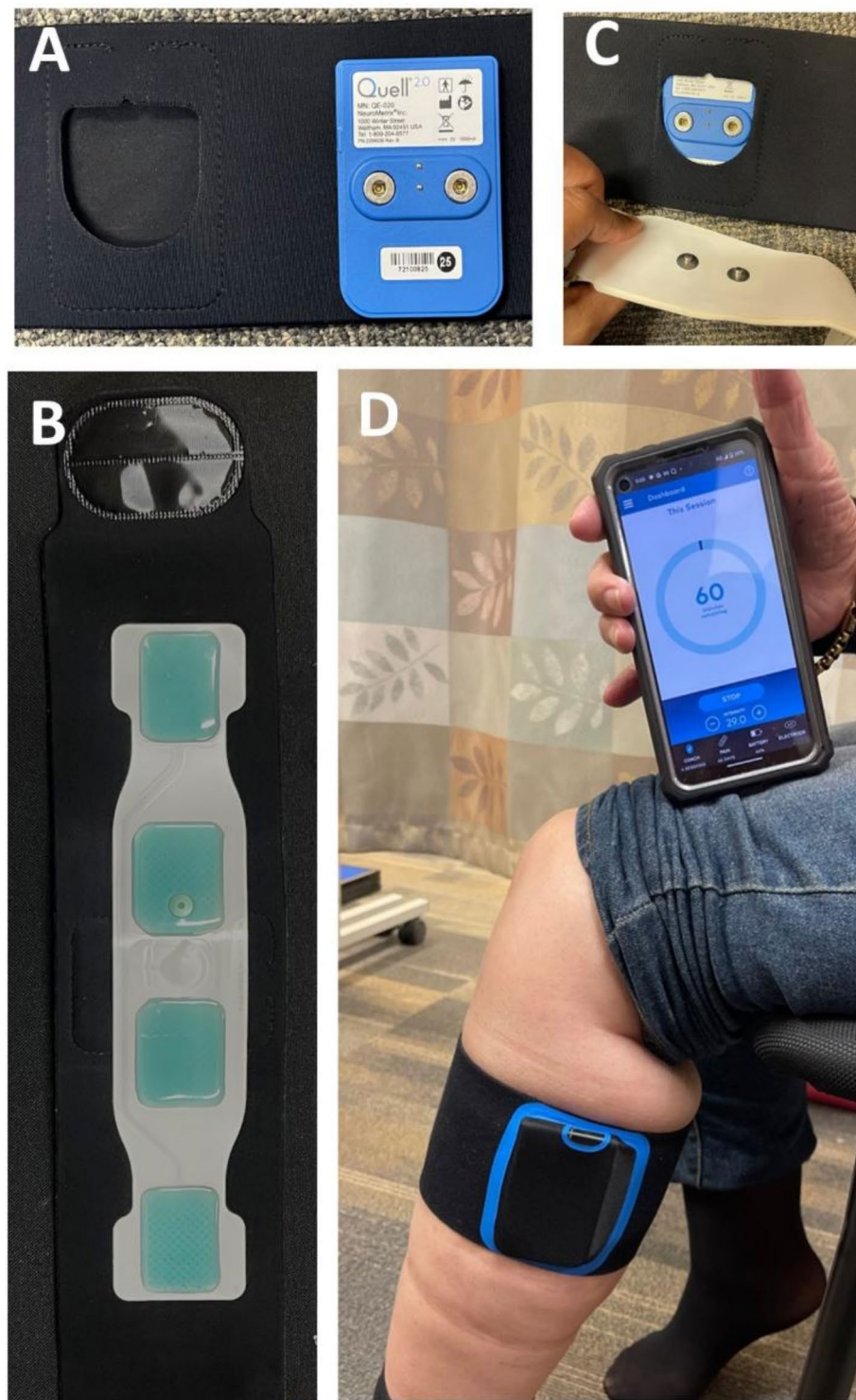
Fig. 1. Transcutaneous nerve electrical stimulation device set up and placement. (A) TENS device located in the band-strap, (B) Hydrogel pad attached inside band-strap, (C) Hydrogel pad connected to the device located inside the band-strap, (D) Band-strap (containing the device and hydrogel) attached around the upper-calf and paired to a smartphone via Bluetooth.
